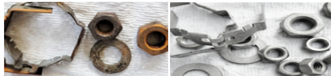
Before high-intensity focused ultrasonic decontamination | After high-intensity focused ultrasonic decontamination
