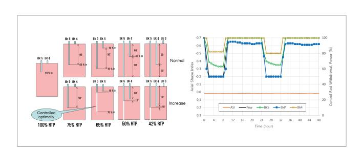
ASI range in low power. Therefore, effective control of ASI is required during low power, which is severely skewed to the top of the core after the middle of a cycle.
