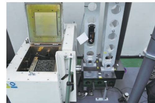
< Weight to Impact and Furnace-1 >
