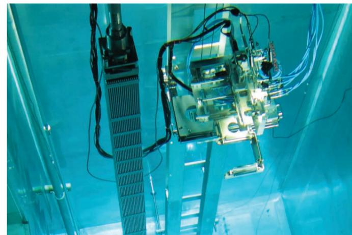
reliability on irradiation performance in the fuel reactor, certifying suitability of fuel rod design code and model and producing irradiation performance data in the indispensable reactor for fuel development.
