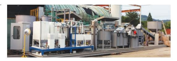
Considering this feature, by physical method, separate micro-soil as well as micro soil, plus the big particle-size one, from the original one to remove only contaminated micro-soil. Therefore, restore uncontaminated soil for the environment by this technology.
